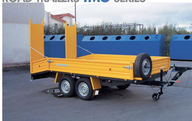
A complete range of homologated **ROAD TRAILERS** with a full load capacity **from 1650 Kg to 3500 Kg,** characterized by a steel frame welded and painted, equipped with inertia brake system with brakes **TUV homologated, adjustable height drawbar, parking jacks and industrial jockey wheel.**
