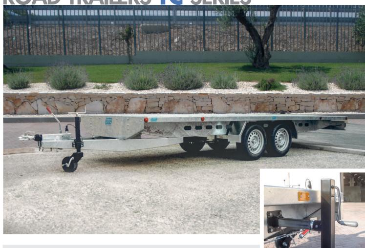
A COMPLETE RANGE OF HOMOLOGATED ROAD TRAILERS, 72 different configurations, all twin axle, full load capacity from 1700 Kg to 3500 Kg. Galvanized steel welded frames, epoxy powder painted as alternative, inertia brake system with brakes TUV homologated.
