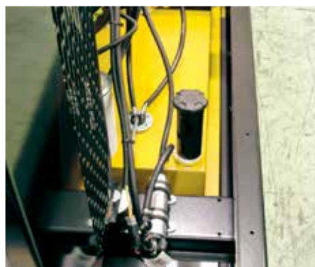
▲ Bunded base system for engine liquids, fuel leaks and acids
