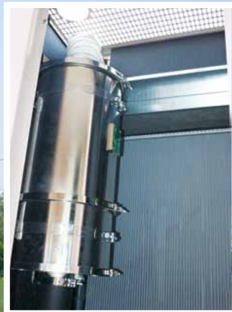
▲ Catalytic anti-particle filter for lower exhaust emissions
