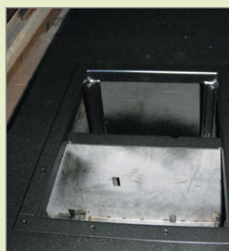
▼ Internal baffles for fuel sloshing control for tanks with capacity > 270 l
