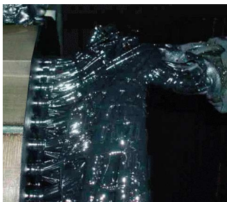
▲ Alternator butadienic protective treatment
